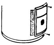
12. Complete wiring to the water heater, or if completed, turn "ON" electric power to the water heater <u>after</u> filling the tank with water.
